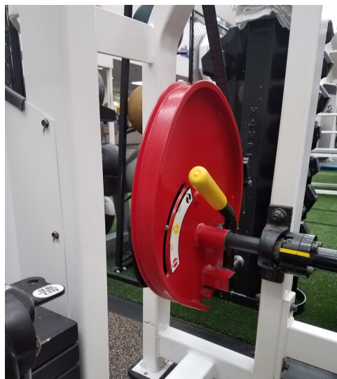
Figure 1: Track on Strive Machines to adjust weight resistance
